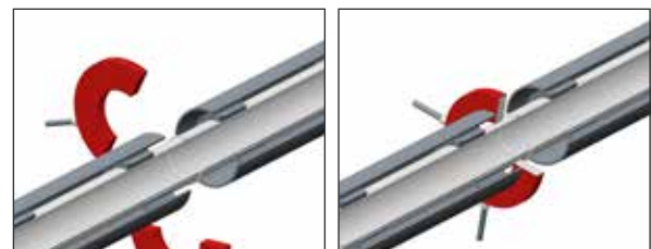
Figure A.16: Step 2: Heating of the outer pipe with a split heating element
