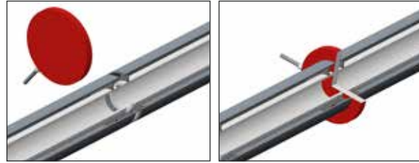
Figure A.9: Step 3: Heating of the joining areas
