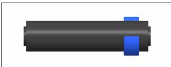
Figure A.26: Step 2: Slide the induction ring onto the pipe
