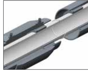
Figure A.12: Inner pipe welded with butt welding
