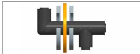
Figure A.20: Step 3: Heating the joining areas
