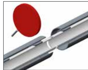
Figure A.15: Step 1: Heating and welding of the inner pipe
