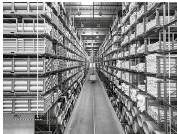
Figure B.2: Horizontal pipe storage
