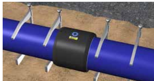
Figure D.20: Fixed welding components
